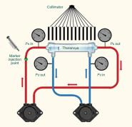
FIGURE 3. The scintigraphic experimental setup. Dialyzer was laid on the gamma camera. Blood (300 mL/min) and dialysate (500 mL/min) were circulated in a closed loop configuration ensuring zero net filtration. The tracer was injected in the blood line, upstream the inlet of the dialyzer. Pressures at inlet and outlet of the 2 compartments were monitored. Pb: pressure blood; Pd: pressure dialysate. Figure adapted from Lorenzin, et al.
