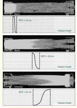
FIGURE 5. MTZ in blood (a, b) and dialysate (c) compartments obtained from the first acquisition. MTZ represents the distance between the point of maximal dye saturation and the point of absolute absence of dye. MTZ: mass transfer zone. Figure adapted from Lorenzin, et al.
