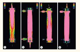
FIGURE 6. On the left, CT images acquired after reaching the total filling in the blood (a) and dialysate (c) compartment in the countercurrent flow experiment. Visible differences are noticed if compared with the same images acquired in the first experiment (b, d). The reduction of dye intensity in the images on the left is the consequence of the internal/backfiltration phenomenon that occurs in countercurrent flow configuration. Figure adapted from Lorenzin, et al.
