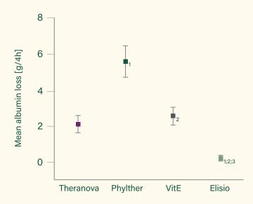
**FIGURE 4.** The mean albumin loss during a 4 h simulated treatment with bovine blood. The flow rate was set to QB=300 mL/min, QD = 500 mL/min, and UF = 10 mL/min. (1) is tested vs. Theranova, (2) vs. Phylther, (3) vs. VitE with p<0.05.
