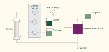
$\ensuremath{\textbf{FIGURE 1.}}$  Experimental setup for the plasma clearance and albumin loss measurements.
