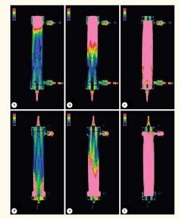
FIGURE 4. Dye progression in blood (a, b, c) and dialysate (d, e, f) compartments after 4 and 12 seconds and at total filling (33 seconds for blood and 28 seconds for dialysate), for the first experimental setup. Blue/green areas are free from dve solution. pink areas point out the presence of the dye solution, and red/vellow areas are transition zones. Figure adapted from Lorenzin, et al.
