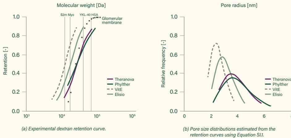
**FIGURE 2.** Solute transport characteristics of the 4 investigated dialyzers. Retention of the glomerular membrane taken from Axelsson et al. (2009). The VitE membrane results need to be taken with care as membrane drying might have affected the pore structure.
