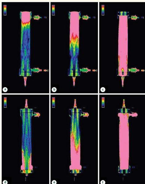
**FIGURE 4.** Dye progression in blood (a, b, c) and dialysate (d, e, f) compartments after 4 and 12 seconds and at total filling (33 seconds for blood and 28 seconds for dialysate), for the first experimental setup. Blue/green areas are free from dye solution, pink areas point out the presence of the dye solution, and red/yellow areas are transition zones. Figure adapted from Lorenzin, et al.
