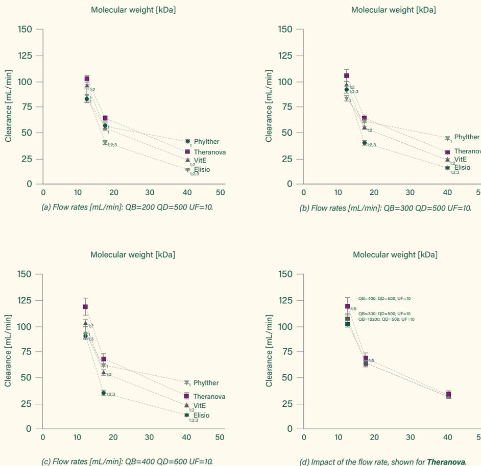
**FIGURE 3.** Plasma clearance data for different middle molecules (82 microglobulin (12 kDa), myoglobin (17 kDa) and YKL-40 (40 kDa)), dialyzer types and flow rate configurations. (1) is tested vs. **Theranova**, (2) vs. Phylther, (3) vs. ViE21X with  $p < 0.05$ . (4) is tested vs. QB=200; QD=500; UF=10 and (5) vs. QB=300; QD=500; UF=10 with  $p < 0.05$ .
