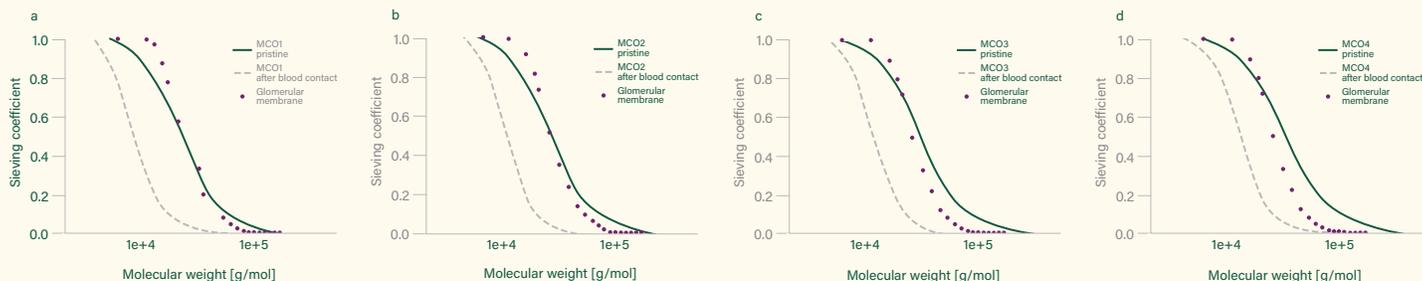
**FIGURE 2.** Characteristics of sieving curves for MCO high flux membranes before (solid line) and after blood contact (dashed line), for (a) MCO 1, (b) MCO 2, (c) MCO 3, (d) MCO 4. The data for the glomerular membrane has been added for comparison (rat specimen, ficoll filtration, measured in vivo).
