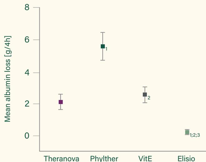
**FIGURE 4.** The mean albumin loss during a 4 h simulated treatment with bovine blood. The flow rate was set to  $QB=300$  mL/min,  $QD = 500$  mL/min, and  $UF = 10$  mL/min. (1) is tested vs. Theranova, (2) vs. Phylther, (3) vs. VitE with  $p<0.05$ .
