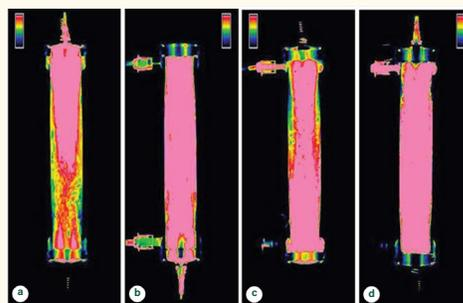
**FIGURE 6.** On the left, CT images acquired after reaching the total filling in the blood (a) and dialysate (c) compartment in the counter-current flow experiment. Visible differences are noticed if compared with the same images acquired in the first experiment (b, d). The reduction of dye intensity in the images on the left is the consequence of the internal/backfiltration phenomenon that occurs in counter-current flow configuration. Figure adapted from Lorenzin, et al.
