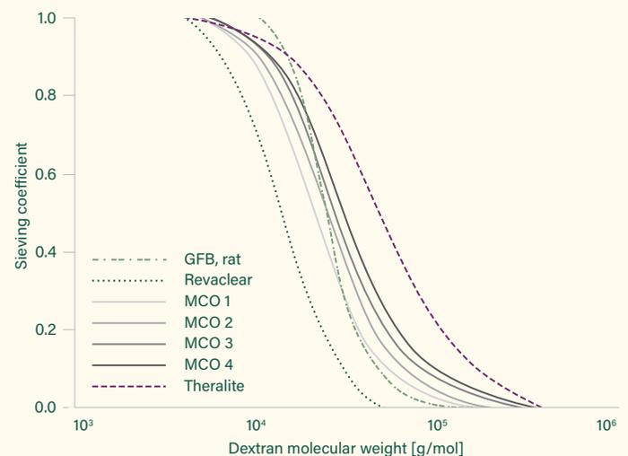
**FIGURE 1.** Characteristic in vitro dextran sieving curves measured in aqueous solution (pristine/before blood exposure) for different types of blood purification membranes: high-flux (Revaclear, MCO membranes 1-4), HCO (Theralite). Data for glomerular membrane added for comparison (rat specimen, ficoll filtration, measured in vivo). Adapted from Boschetti-de-Fierro et al.
