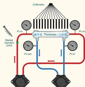
**FIGURE 3. The scintigraphic experimental setup.** Dialyzer was laid on the gamma camera. Blood (300 mL/min) and dialysate (500 mL/min) were circulated in a closed loop configuration ensuring zero net filtration. The tracer was injected in the blood line, upstream of the inlet of the dialyzer. Pressures at inlet and outlet of the 2 compartments were monitored. Pb: pressure blood; Pd: pressure dialysate. Figure adapted from Lorenzin, et al.
