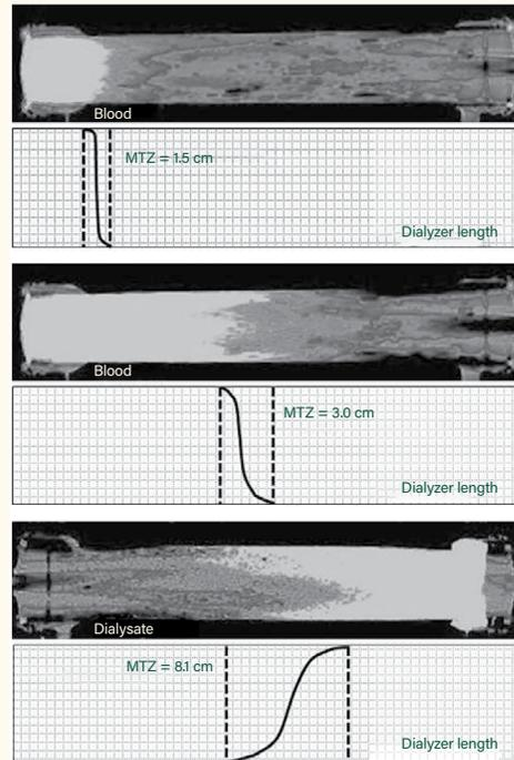
**FIGURE 5.** MTZ in blood (a, b) and dialysate (c) compartments obtained from the first acquisition. MTZ represents the distance between the point of maximal dye saturation and the point of absolute absence of dye. MTZ: mass transfer zone. Figure adapted from Lorenzin, et al.
